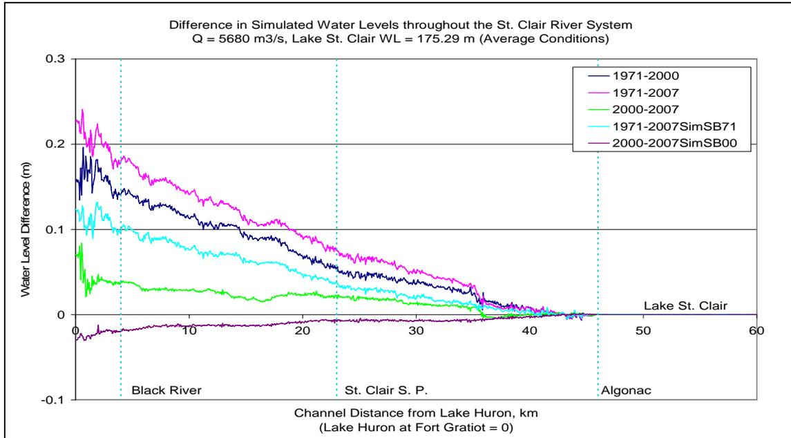
**Figure 6: Difference between water surface profiles generated for various years (e.g. “1971 - 2000” is equal to the 1971 water surface elevation minus the 2000 water surface elevation at points along the river centerline).**
