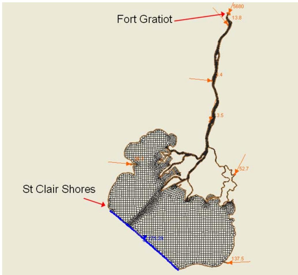
Figure 4: Model mesh extent and boundary conditions (discharge boundaries shown in orange with arrows, water level boundaries shown in blue with line and triangle).
