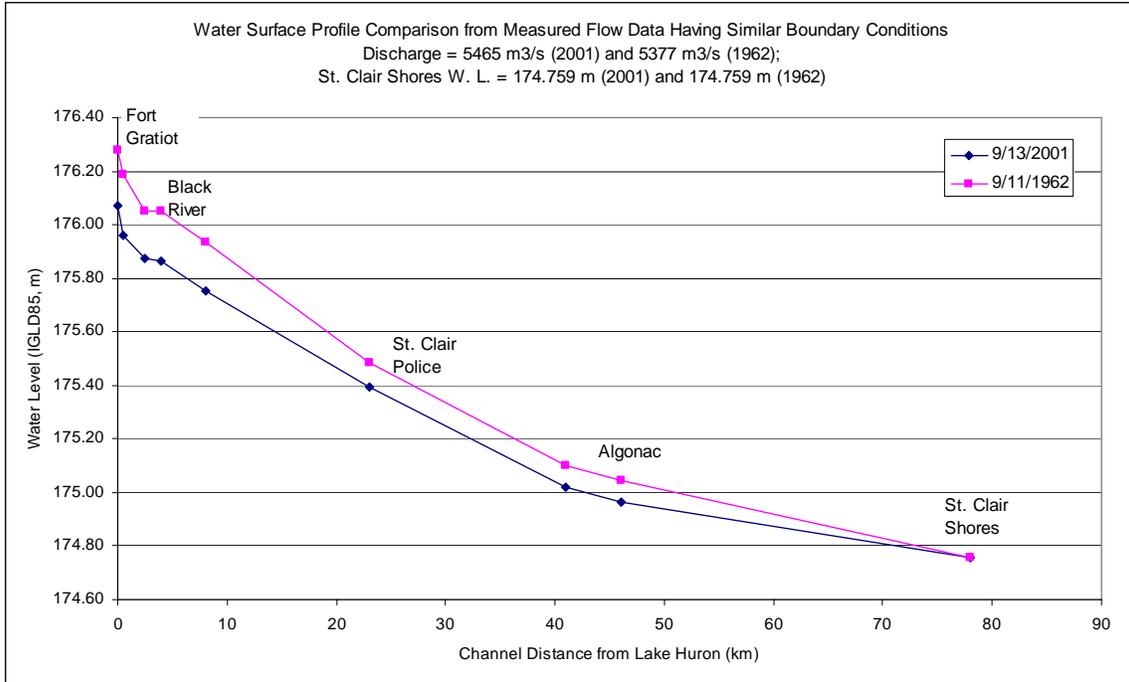
**Figure 2: Example of water surface profiles having similar boundary conditions (Figure 6-5 from Bruxer, 2009). Fort Gratiot difference is approximately 20 cm.**
