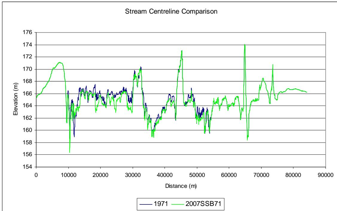
**Figure 1: Stream centerline comparison of bed surfaces from 1971 and 2007 simulated single-beam (2007SSB71) model.**
