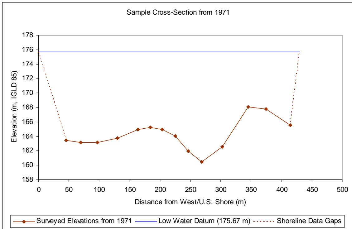
Figure 8: Sample cross-section from 1971 showing the surveyed elevation points, the Low Water Datum, and the assumption made regarding the elevation of the near-shore areas.
