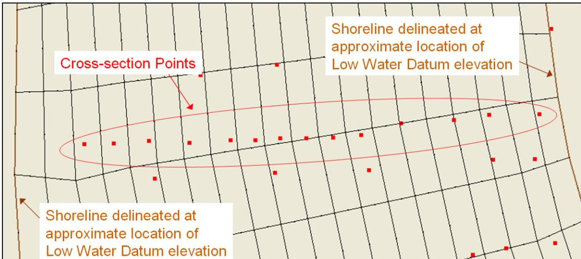
Figure 7: Illustration of sample cross-section surveyed points from 1971, plus model shoreline, which was delineated at the approximate location of the Low Water Datum elevation.
