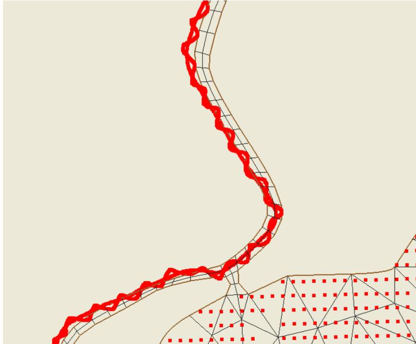
Figure 5: Example of model mesh (black grid with brown outline) and bathymetry data (red dots and “lines”) for Chenal Ecarte not coinciding.
