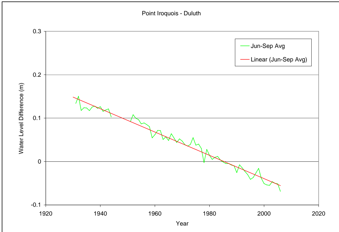
Figure 3-1: Water level difference plot of Point Iroquois minus Duluth (Lake Superior). Water levels were averaged from June to September in this case.
